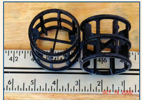
Bacteria attaches itself to thousands of these media in the Biocon chamber where active digestion results in reduced pollutants, including phosphates and nitrates.
