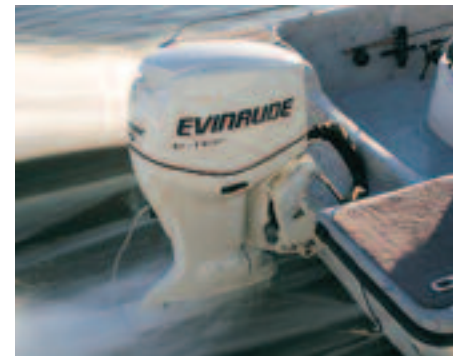
An E-Tec 90 hp outboard motor is an example of the new direct, fuel-injected two-stroke engines.
